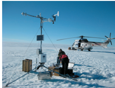
GEUS constructed and manage a network of climate stations to monitor the ice sheet.
