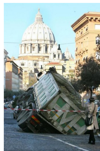
Fig. 2 - A sinkhole opened in a street of Rome ( www.roma.repubblica.it ).
